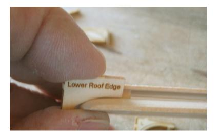
Shaping of the lower roof is the first step. The templates are clearly marked and need to be sanded with a finger nail board until the suitable profile is obtained. As passenger car roofs are more square than trolley roofs, the finished appearance will vary between the two types of cars. At the inner edge, where the roof extension board is concerned, this shape is nearly identical for both models.
