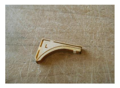
Identify the suitable roof extension piece for each location on the roof. Here is an example using the left. Visible is the trace line that will ultimately be the upper shape of the roof line. Below offers a very prototypical appearance of the hollow area as the upper roof curves down to the lower. All of the material above the trace line will be sanded away during final finishing.
