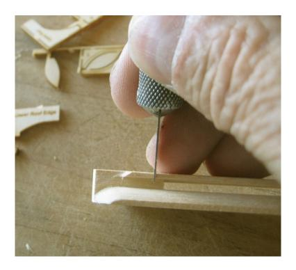
Visible now is the shaped lower roof and the clearing of the upper roof overhang to make way for the curved insert piece. The knife is cutting back to the end of the insert piece.
