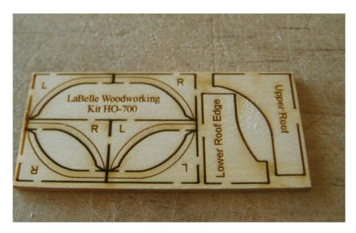
Shown here, a #700 passenger jig kit as supplied from the manufacturer. At the right are the profile shapes for the rounding of the roof ends. At the left are the four pieced necessary to extend the clerestory overhang down to the roof end.
